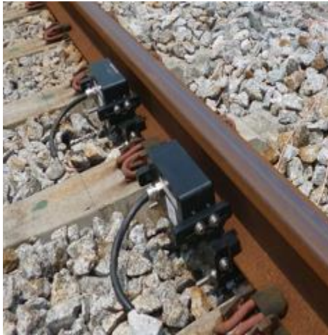
Figure 1. Electromagnetic sensors embedded in a railway track.
