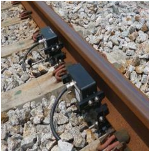
Figure 1. Electromagnetic sensors embedded in a railway track.
